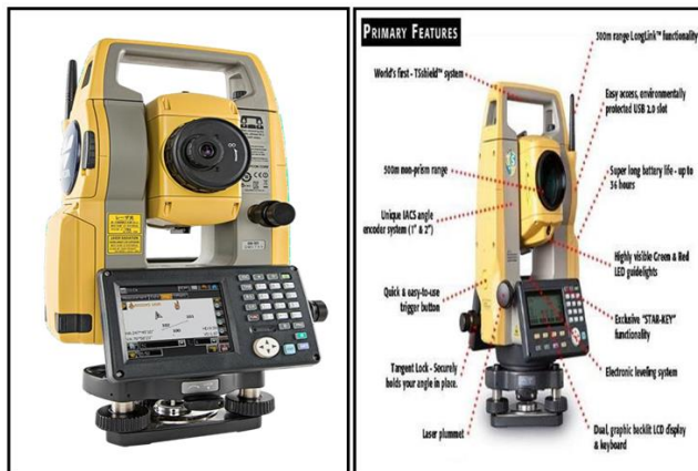
Gambar 24. Total Station (a): Bagian-bagian Alat Total Station (b)
